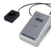
1 sun checker is used for checking the light intensity (1 sun) of HAL-320. It is battery operated and portable.
