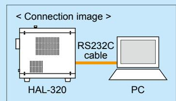
The HAL-320 can be controlled remotely via RS232C.
