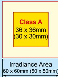
The values shown in parenthesis are the values of illumination at the recommended size. In this case, it needs to check the light intensity separately.
