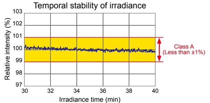
\*10 minutes measurement after turning on the lamp for 30 minutes.
