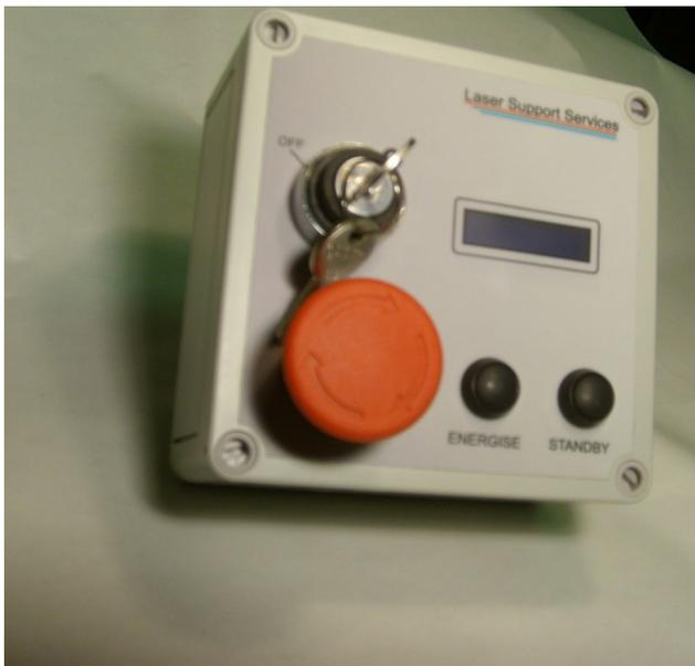
As the name implies the MCU controls all the functions of the system, the easy to read LCD states current status and also indicates, should a problem arise, which door it is on.
