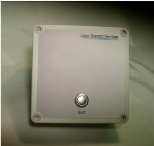
The DCU controls the door where it is located, communicating the status of the door switches and the magnetic locks back to the MCU.
